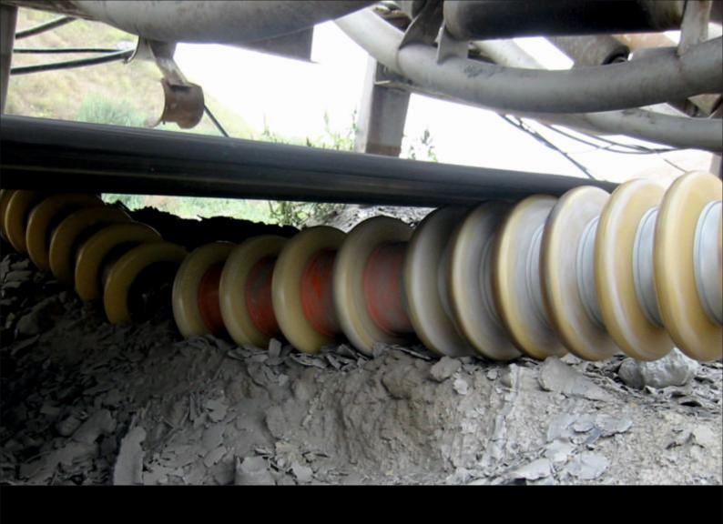
Our polyurethane wheels are rolling the conveyor belts of mining sites worldwide. We have manufactured and supplied the mines with more than 2.500.000 wheels and this quantity keeps increasing from day to day. We work one to one with our customers bringing solutions to the mines and delivering top quality parts designed to provide the best overall performance and longest lifespan.
